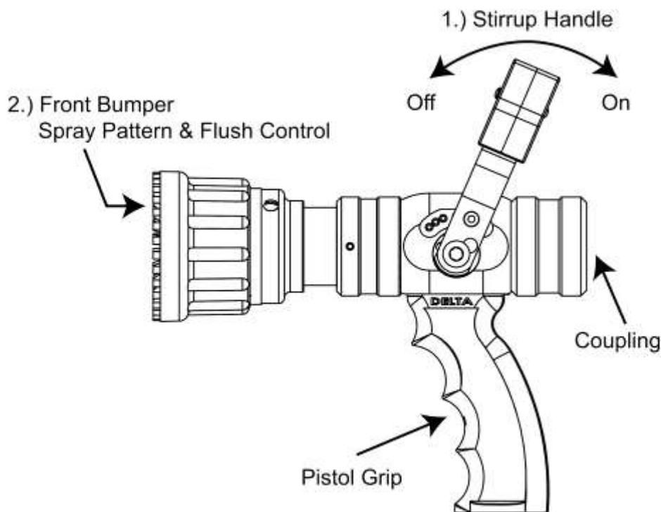
The H500 Nozzle has full water stream pattern control, from straight stream to wide spray/fog settings, fully adjustable by simple rotation of the front bumper. An additional 'flush' setting is available by counter-clockwise rotation of the bumper to enable the operator to clear debris that may have entered the nozzle inlet via the water stream.
